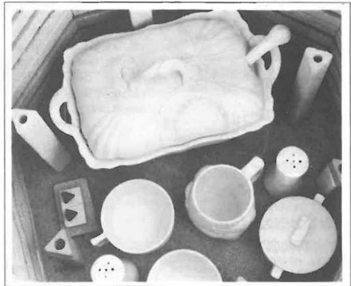
Two sizes of greenware loaded directly on kiln's floor. Note different sizes of posts and use of two large pyrometric cones behind the peephole.
