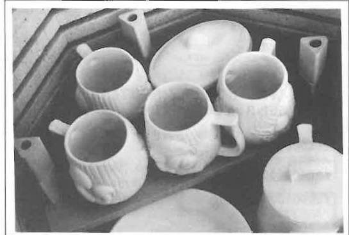
Shelves placed on posts and ware loaded. Note ware to be used together should be fired together in the greenware firing.
