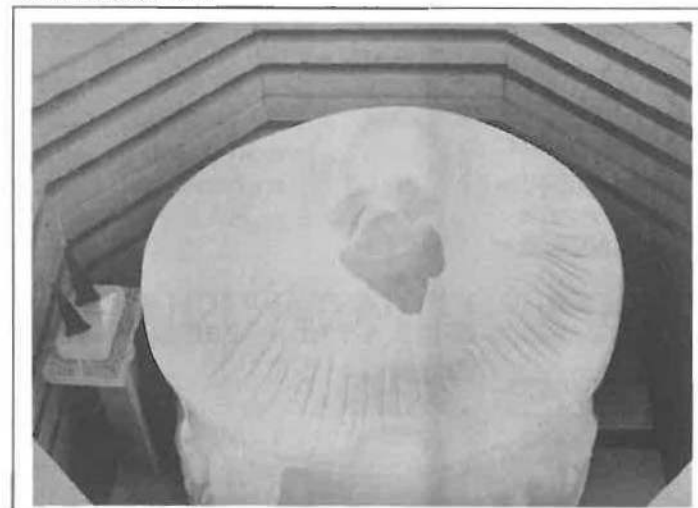
Large, heavy pieces of greenware will fire best if placed across two half shelves positioned at an even height.
